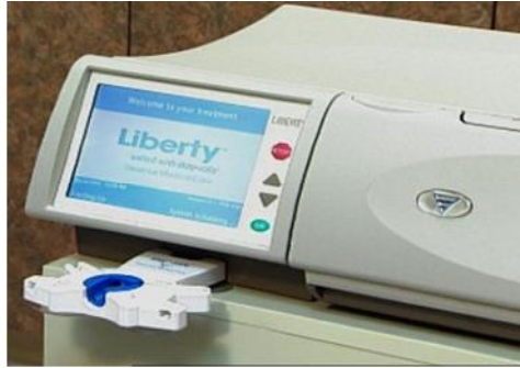
FIGURE 6. The Liberty Cycler. The cycler pumps dialysate (a cleansing solution used to draw waste products and extra fluids out of the blood) into the empty peritoneal cavity. There it absorbs waste through the body's natural membrane over a set amount of time [14].
